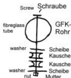
how to prepare the fibre tubes
